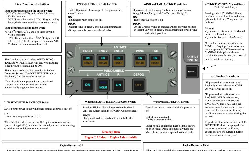
When anti-ice is used during ground operations in icing conditions, perform an engine run -up of 60% N1 for 30 seconds prior to takeoff. This run -up should also be performed if anti-ice is used during ground operation for any period greater than 30 minutes, and repeated at intervals of no greater than 30 minutes.
